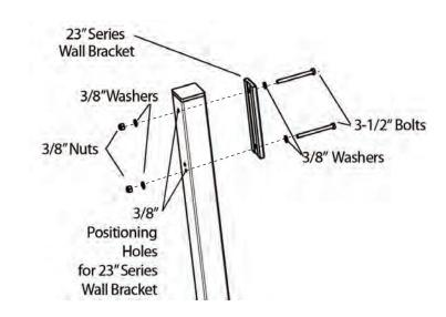
Figure 4 Pole Mount Configuration for 23" Series
